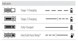
\*The red light will continue to blink, but a yellow indicator light will be illuminated during this operation. Once the battery pack has reached an appropriate temperature, the yellow light will turn off and the charger will resume the charging procedure.
