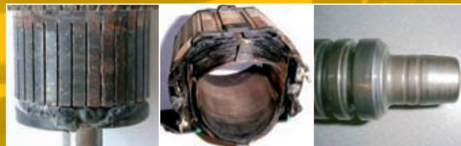
Melted end piece - overloaded Melted field terminals Worn beatpiece
