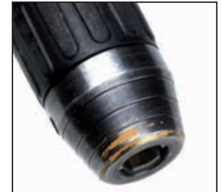
Wear caused by operating the drill with the chuck running against masonry or other hard surfaces
