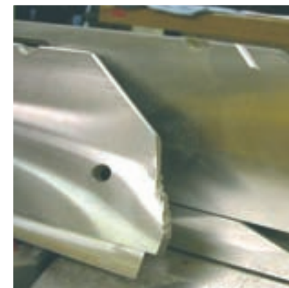
Abused fence - blade impact
