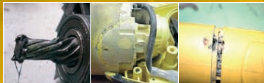
Pinion wear Extreme contamination / residue Damage caused by polishing activity with grinders
