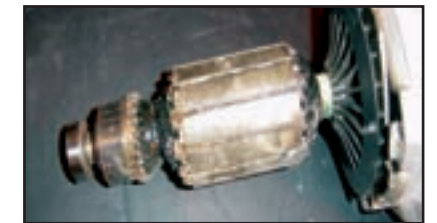
Armature burnt out (overloaded)
